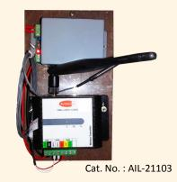
The Transmitter which will be installed in each equipment whose data is to be shown in the Central Monitoring System.
